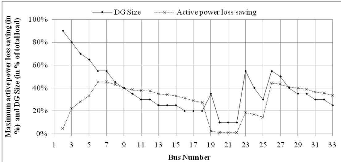
Fig. 7: Maximum active power loss saving and corresponding size of UPF DG at different buses of 33-bus system
