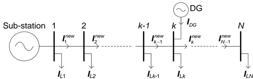
Fig. 2: A typical N-bus radial distribution system with DG placed at bus k
