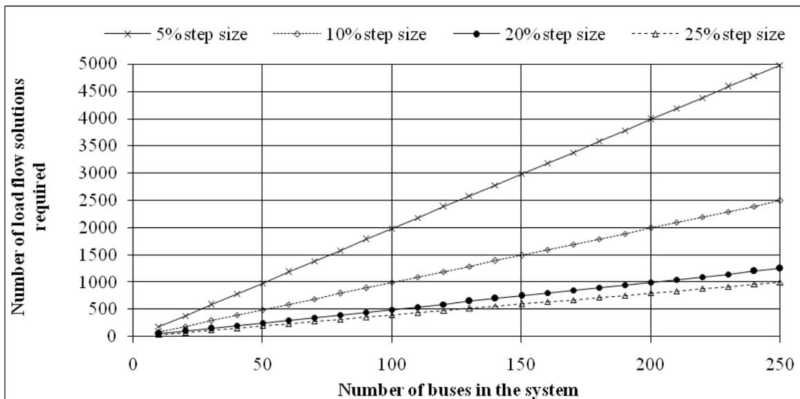
Fig. 17: Variation in number of load flow solutions required with system size and incremental step-size for DG
