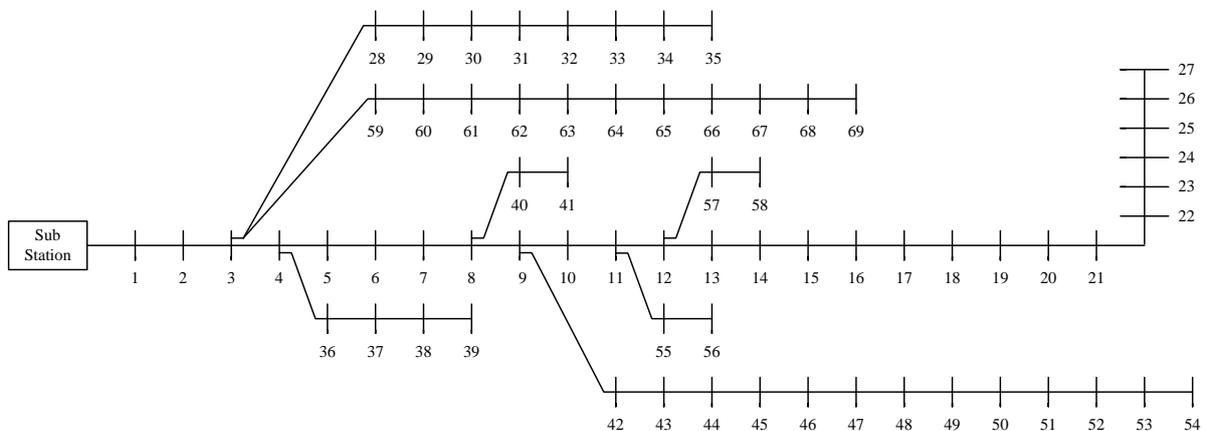
Fig. 10: Single line diagram of 12.66 kV, 69-bus distribution system
