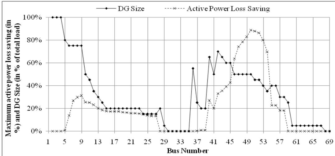
Fig. 11: Maximum active power loss saving and corresponding size of LPF DG at different buses of 69-bus system
