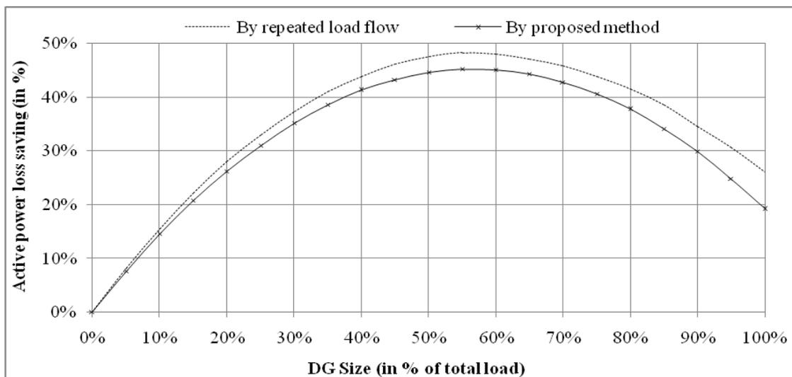
Fig. 8: Comparison of active power loss saving with UPF DG connected at bus 6 of 33-bus system
