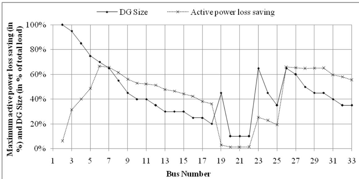
Fig. 4: Maximum active power loss saving and corresponding size of LPF DG at different buses of 33-bus system
