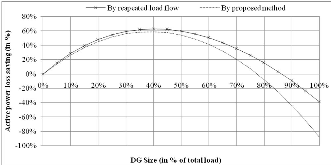
Fig. 15: Comparison of active power loss saving with UPF DG connected at bus 50 of 69-bus system
