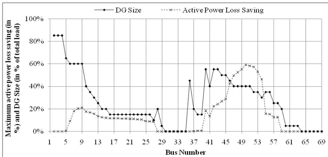
Fig. 14: Maximum active power loss saving and corresponding size of UPF DG at different buses of 69-bus system
