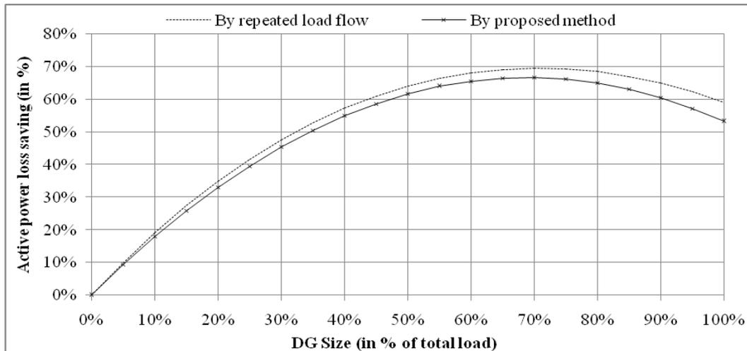
Fig. 5: Comparison of active power loss saving with LPF DG connected at bus 6 of 33-bus system
