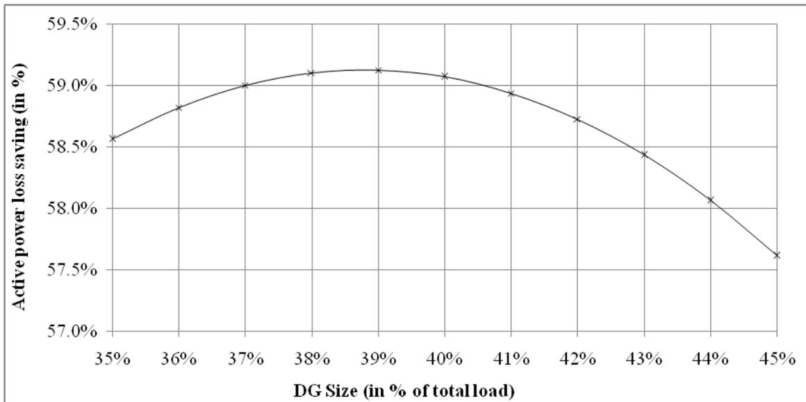
Fig. 16: Active power loss saving with UPF DG connected at bus 50 of 69-bus system
