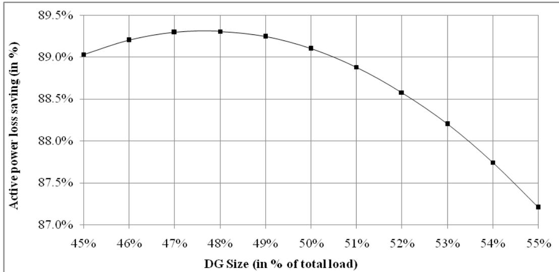
Fig. 13: Active power loss saving with LPF DG connected at bus 50 of 69-bus system
