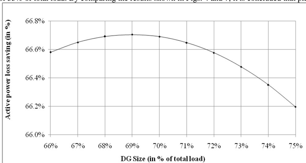
Fig. 6: Active power loss saving with LPF DG connected at bus 6 of 33-bus system
