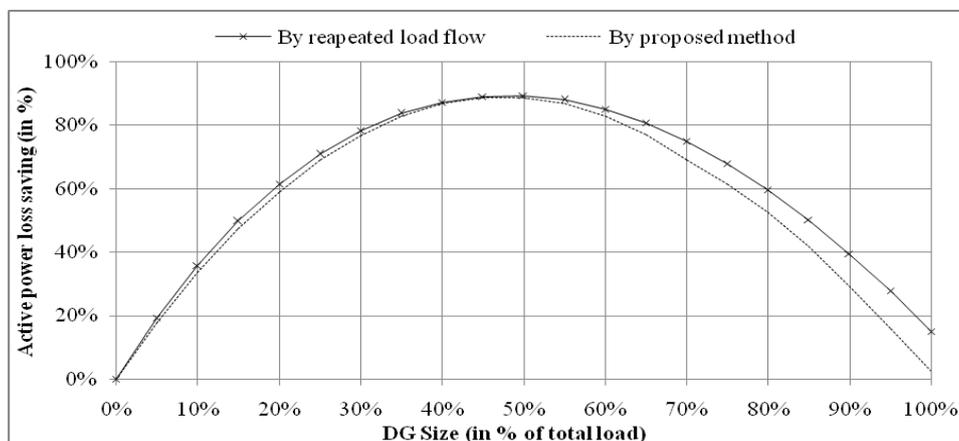
Fig. 12: Comparison of active power loss saving with LPF DG connected at bus 50 of 69-bus system
