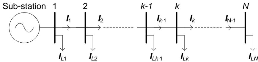
Fig. 1: A typical N-bus radial distribution system
