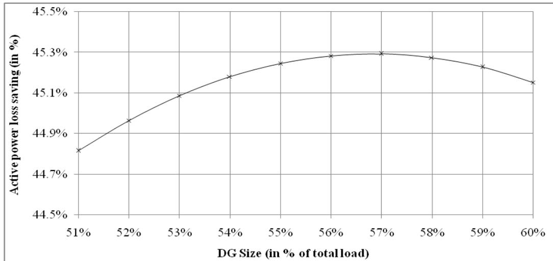
Fig. 9: Active power loss saving with UPF DG connected at bus 6 of 33-bus system
