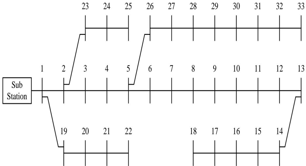
Fig. 3: Single line diagram of 12.66 kV, 33-bus radial distribution system
